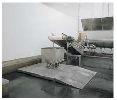
Correct positioning of the ProDec speeds up work flow. Place ramps on one, two, three, or four sides to create optimum traffic patterns.
