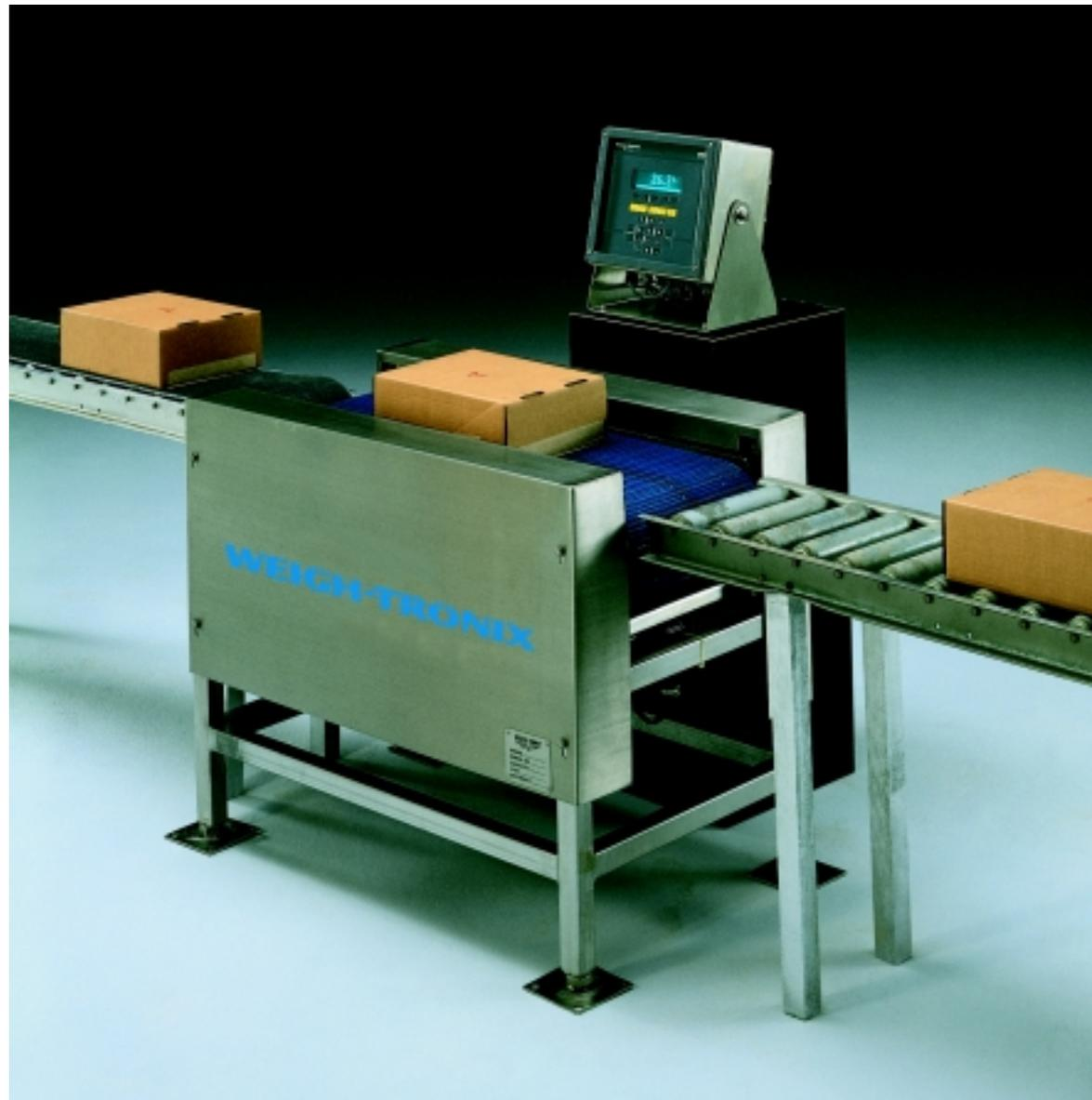
The Weigh-Tronix conveyor scale is a freestanding, self-contained and self-powered, flat-belt weighing system that can be incorporated into new or existing production facilities. The scale operates while the conveyor is in motion and is intended for the weighing of individual boxes, cartons, cans or unpackaged products such as large cuts of meat. It is ideally suited to checkweighing, straight weighing and weight accumulation operations.
