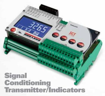
For PLC systems that require weight data from a scale, Rice Lake's SCT transmitters deliver signal conditioning in a compact design. SCT models are DIN-rail mountable within a cabinet or control panel, where they convert a scale's load cell signal to a digital signal that can be sent via serial, analog or network protocol outputs. Choose between the SCT-10, SCT-20, SCT-30 or SCT-40.
