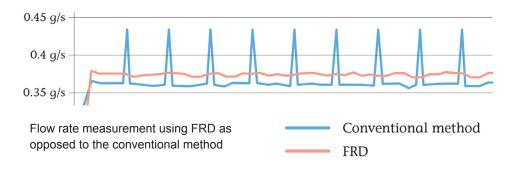
\*1 Flow rate is determined from the weight variation that occurs during a given interval.
