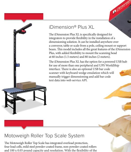
iDimension Plus XL, you can pair together to help improve the process of your existing workflow. Dimension and weigh each package in less than 1 second.
